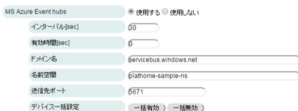
The image shows a configuration form for MS Azure Event hubs. It includes a title bar with a radio button for '使用する' (checked) and '使用しない'. Below are several input fields: 'インターバル[sec]' with value '60', '有効時間[sec]' with value '0', 'ドメイン名' with value 'servicebus.windows.net', '名前空間' with value 'plathome-sample-ns', and '送信先ポート' with value '5671'. At the bottom, there are two radio buttons for '一括有効' and '一括無効'.
